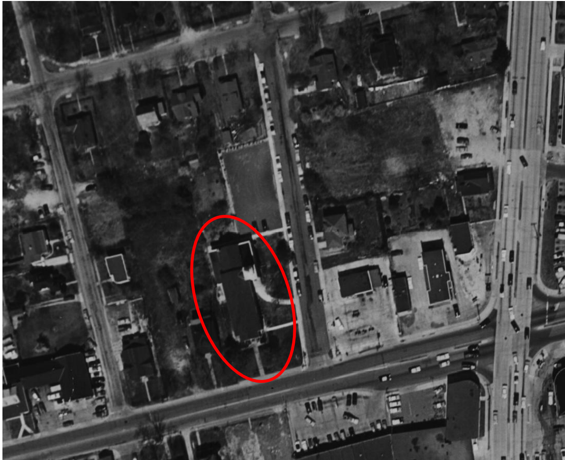
Figure 52: Aerial of Arlington Presbyterian Church, 1956. The photograph shows the renovations completed in 1950. Visible alterations include: 1) demolition of original lantern and spire; 2) construction of new steeple in the northeast corner of the building; and 3) construction of rear addition.
